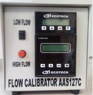
Device under calibration need to be connected at inlet of the calibrator
